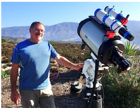
The telescopes and ccd cameras that John uses to monitor the dimming of faint stars.
