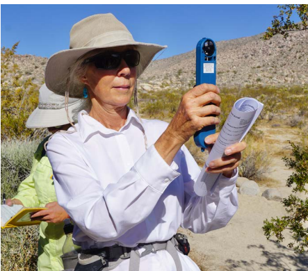
Lisa Pridmore uses the Ambient Weather WM-3 which can measure wind speed, temperature, humidity, wind gust and Beaufort Scale.
