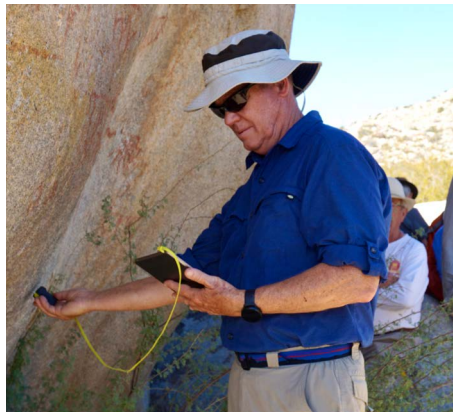
Neil Cadwallader checks the surface humidity of the rock face that is displayed on an iPad.
