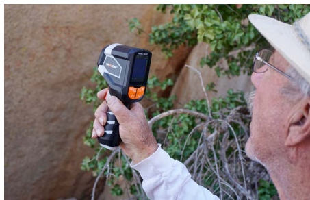
Chuck Bennett uses the Maka thermal imager to measure surface temperature of the rock.
